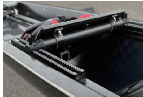
"Shark tooth" stretcher tracks system
